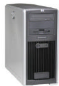
xw8000 4Gb dual Xeon 375Gb storage Serves as Workstation, data backup, webserver
